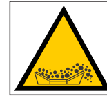
SWW 21 WRN FALLING MATERIAL FROM CONVEYOR
