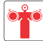
SFB 8 FIRE PUMP CONNECTION
