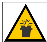
SWW 48 WRN HOT MATERIAL IN CONTAINER
